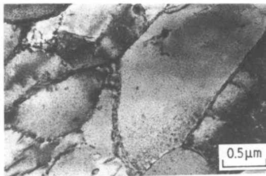
Figure 3 TEM view of specimen aged at 110° C for 192 h.
